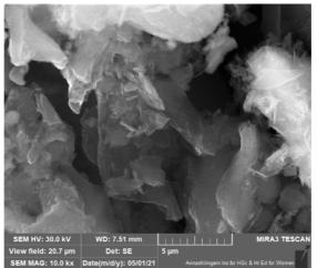
Fig.3. SEM, analysis of *Cassia absus* seed mediated CuNPs
