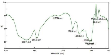
Fig.2 FTIR analysis of Cassia absus seed mediated a) CuNPs b)CuNPs
